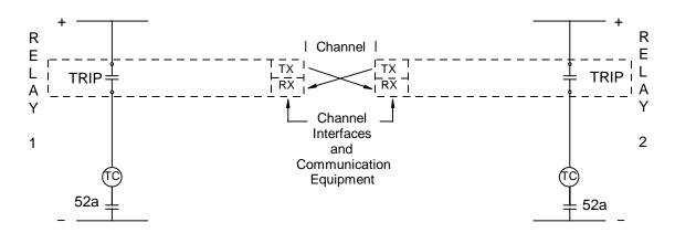
FIGURE 3. DIRECT RELAY-TO-RELAY DIGITAL LOGIC COMMUNICATION
