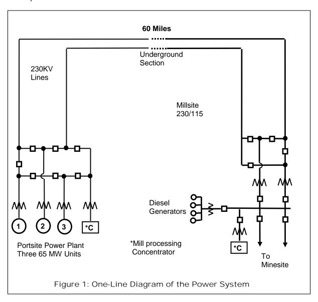
With a dependable communications network in place, the primary and secondary protection systems for the parallel 230 kV lines could be selected to provide as much redundancy and reliability as possible. The two systems were made by different vendors and operate on different principles in order to minimize the risk of common mode failures. The primary
