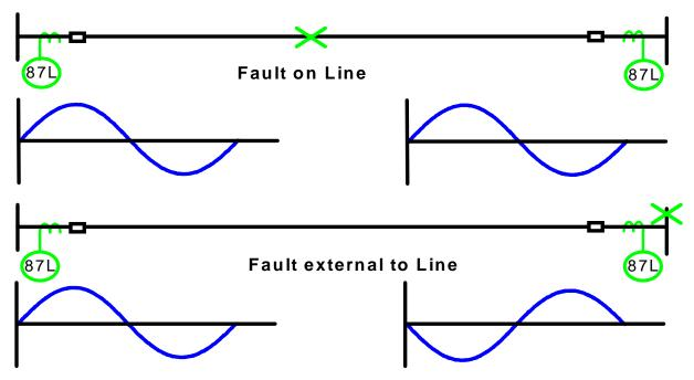
Figure 2: Segregated Phase Comparison Signals
