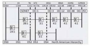
the DS1 1.544 Mbps and SONET overhead bits. Single-step multiplexing up to STS1 requires no bit stuffing, and VT's are easily accessed.
