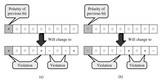
Figure 7. Bi-polar with 8-zero substitution (B8ZS)
