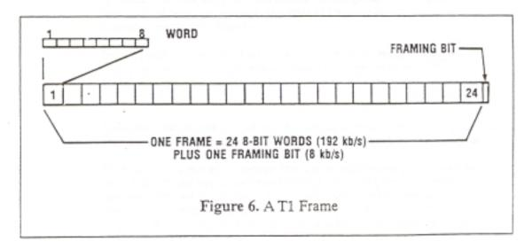
Since the DS-0 signals are sampled 8000 times per second, it means that 8000 192-bit information frames are created during that period. Total: 1.536 Mb/s. At 8000 samples per second, framing bits are created at the rate of 8 kb/s. Result: A single 1.544 Mb/s signal known as digital signal-level one (DS-1).
