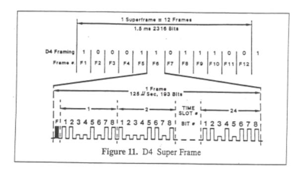
Table 1 outlines the superframe format as stated in ANSI standard T-1.403-1989. As previously stated a superframe is made up of 12 individuals frames, with the 193rd bit in each frame used as a control bit. When combined, these control bits form a 12-digit word (100011011100) that provides frame and signal management.
