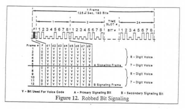
Using robbed bit signaling, the least significant (8th) bit of the DS-0's in the 6th and 12th frames is reserved for signaling information. The steady state of the bit, 0 or 1, indicates whether the called device is on-hook, off-hook, disconnected, busy, etc.
