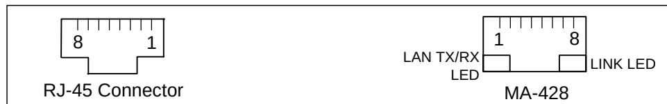
Figure 15. Pins 1 and 8 on RJ-45 connector and on MA-428 LAN Bridge
