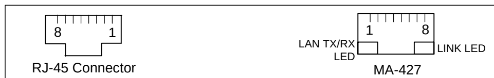
Figure 13. Pins 1 and 8 on RJ-45 connector and on MA-427 LAN Bridge
